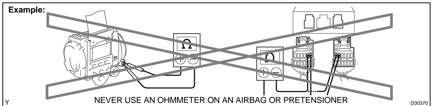
(h) AIRBAG SENSOR ASSEMBLY (ECU)
